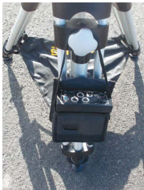
Image 5 - 10Micron's Linux-based computer is purpose designed for unobtrusive control of the GM1000.
