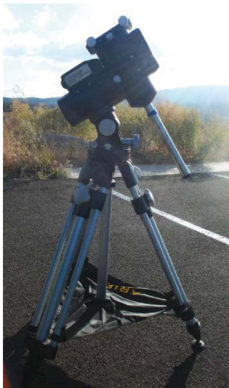
Image 10 - The assembled GM1000 mount and Aries Tripod, ready to accept an imaging scope and camera.
