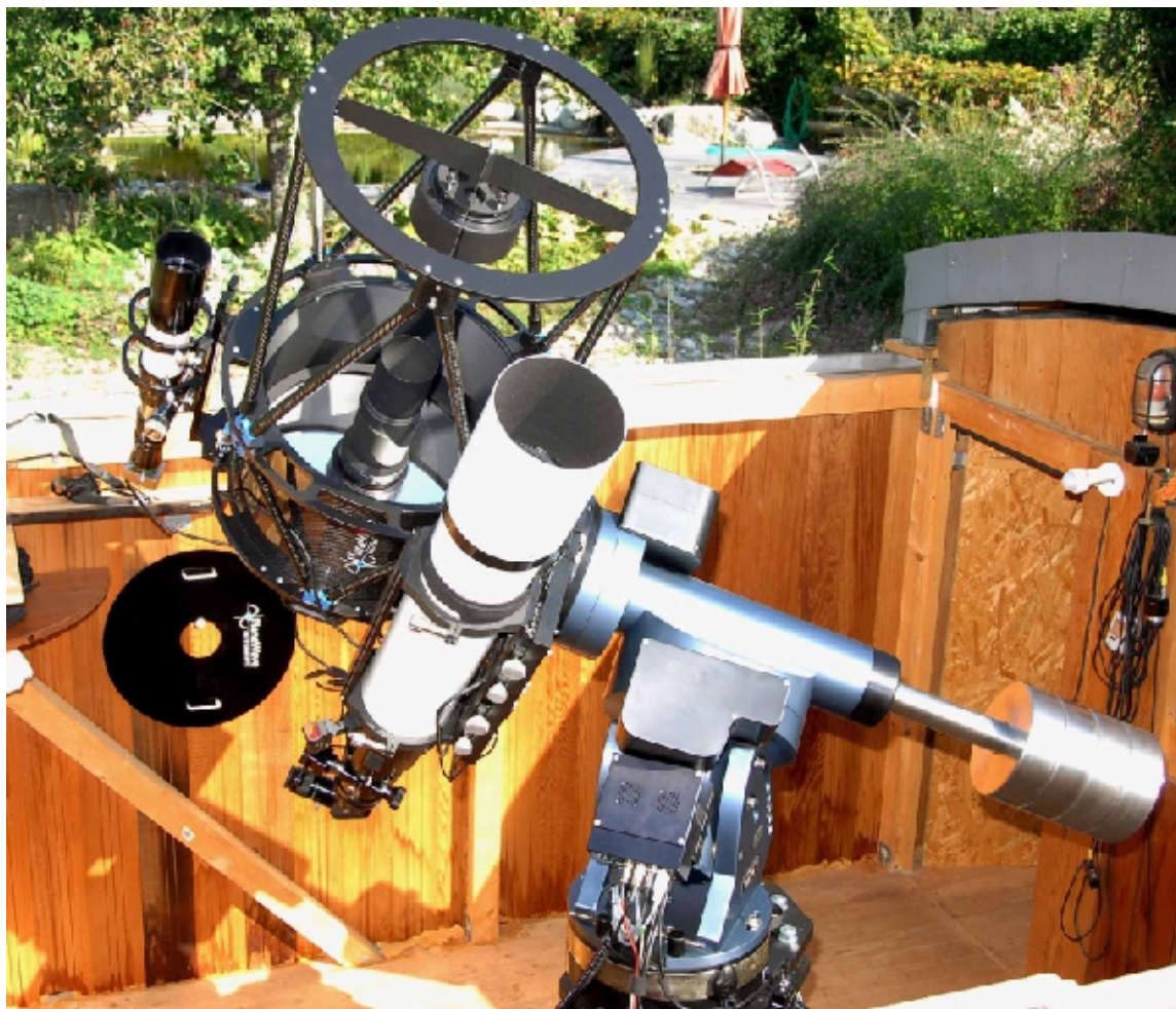
GM4000 mount with Planewave 17" and refractor Astro Physics 155. Each counter weight is 20 kg!
