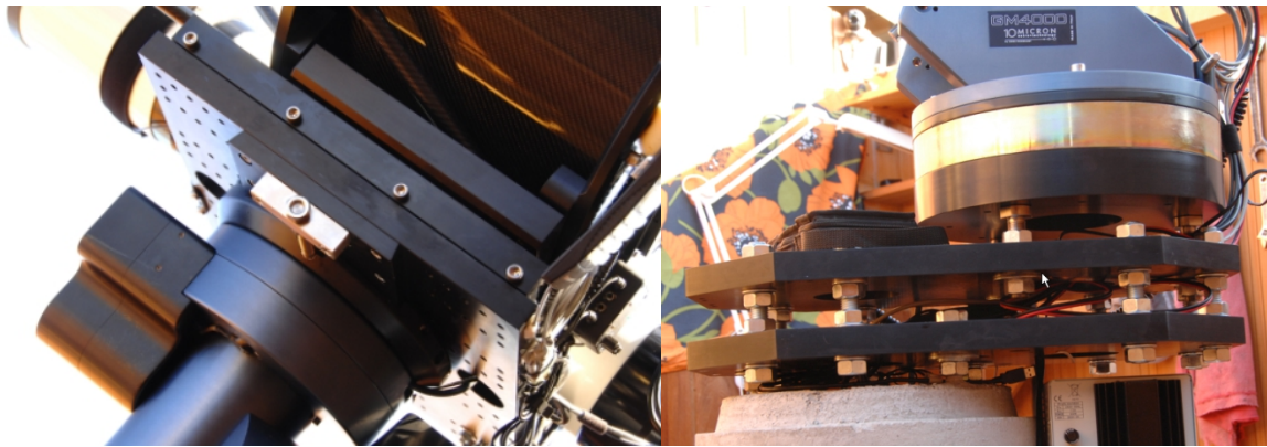
Left: dovetail lateral displacement system. Right: level adjustment system through 3 fine threads.
