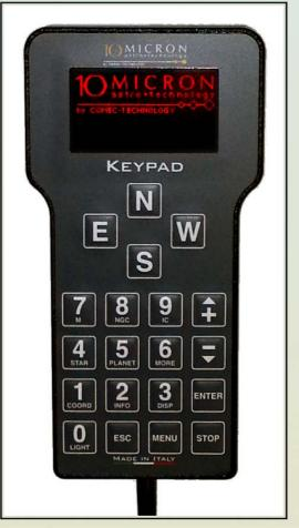
compensated with respect to the stars. You may load orbital elements of comets, asteroids and artificial satellites into the mount, so that these objects can be tracked directly using the keypad (without any external PC).
