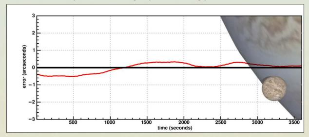
*Tracking error profile measured with an encoder coupled to the r.a. axis. Jupiter and Ganymede are shown as they appear from Earth, at the same scale.*
