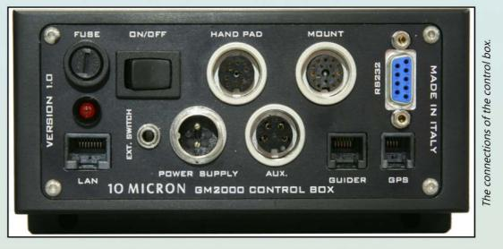
The electronics is housed in an independent control box, easily removable. The connections of the mount and keypad feature secutiry lock screws.
